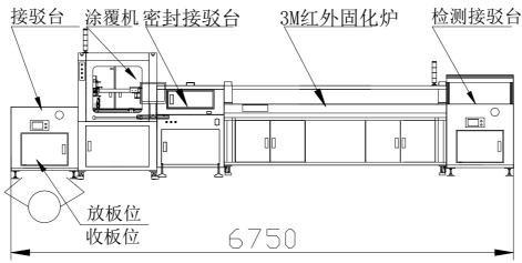
Conveyor----Selective coating machine ZM-830----Sealed Conveyor----3M Curing Oven----Testing Conveyor
